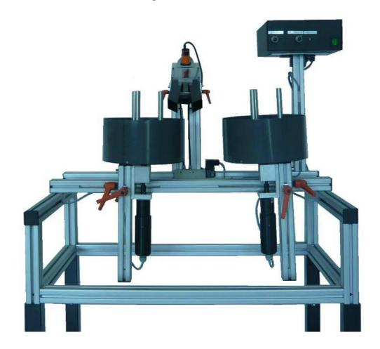
With this double pot-winder, it is possible to coil certain cables and wires to coils. The double pot-winder is available in two versions without motors and with motors. The pot winder is used behind our ISOMAT and Autocut. An installed feeder tube switches over from one pot to the other once one cable is feeded into the pot.
